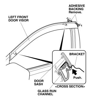
11. Using the palm of your hand, firmly press the left front door visor against the door sash.
