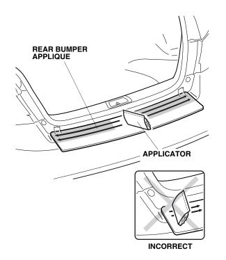
12. Once the flat surface is completely smooth with no bubbles, use the applicator to apply the rear bumper applique to the rounded rear edge at the center as shown.
