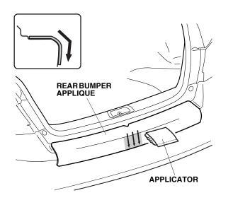
13. Use the applicator to apply the rear bumper applique to the rounded rear edge on the left side as shown. Start in the middle and work outward. Repeat on the right side.
