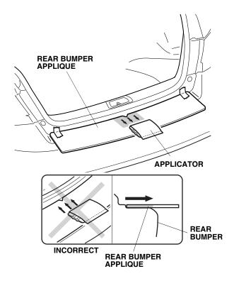
Starting from the center and working outward, use the applicator to smooth the rear bumper applique. Repeat on the right side. Stroke in one direction only.
