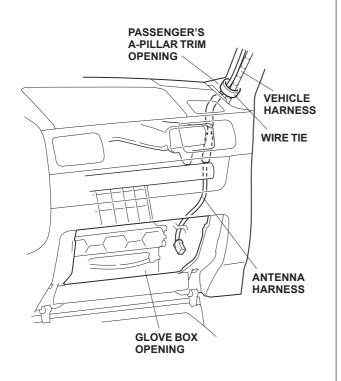
20. Inside the glove box opening, route the antenna harness along the vehicle harness and towards the driver's side of the vehicle. Secure the antenna harness to the vehicle harness with three wire ties in the areas shown.
