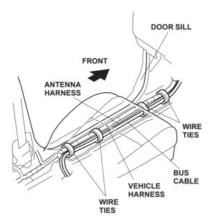
35. Route the bus cable and antenna harness as shown and secure it to the vehicle harness using four wire ties.
