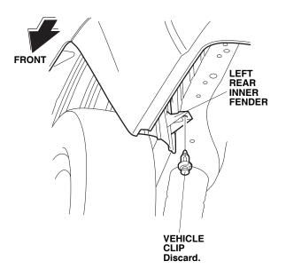
3. While holding the left rear splash guard against the vehicle, secure the splash guard with one clip.
