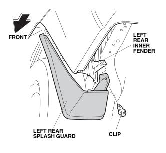
4. Install the left rear splash guard with two self-tapping screws in the order shown. Make sure that there is no space between the rear bumper and the splash guard before tightening the screws.
