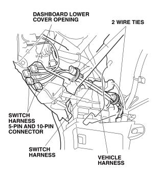
35. Secure the switch harness to the vehicle harness with two wire ties.
