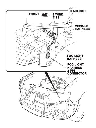
19. Secure the fog light harness to the vehicle harness with two wire ties.
