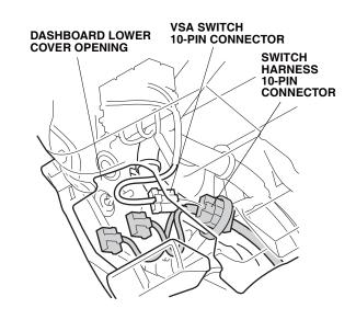
37. Plug the switch harness 5-pin connector (gray) into the fog light switch, and plug the switch harness 10-pin connector (gray) into the vehicle VSA switch.
