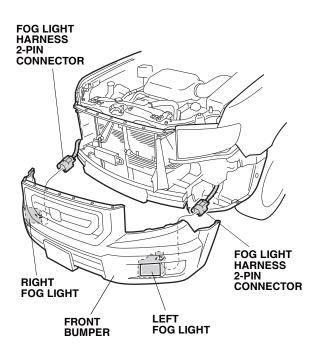
25. Reinstall the front bumper. Have an assistant help you when installing the front bumper.
