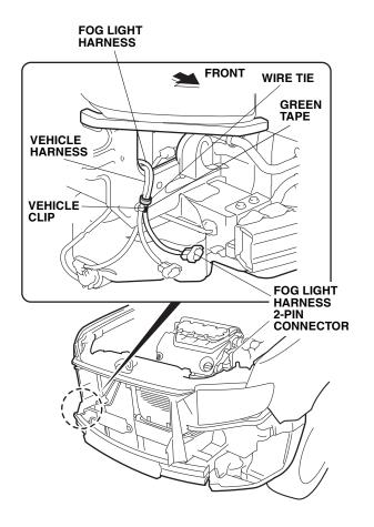
11. Secure the fog light harness to the vehicle harness with one wire tie.
