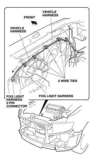
15. Secure the fog light harness to the vehicle harness with five wire ties.
