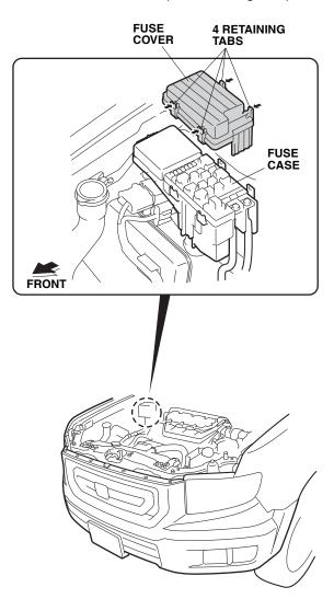
29. Install the fuse (20A) into the fuse case as shown.
