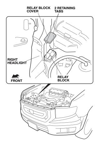
27. Install the relay into the vehicle relay block.
