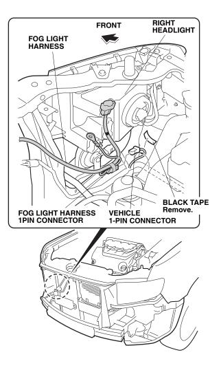
7. Plug the fog light harness 1-pin connector into the vehicle 1-pin connector.
