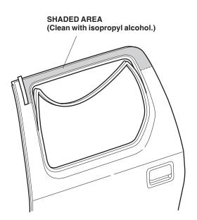
Attach a strip of the masking tape to the ends of the long adhesive backings, and remove 2 to 3 in. (5 to 8 cm) of adhesive backings. Fold back the ends, and tape the ends to the front of the door visor. Remove the short adhesive backing.
