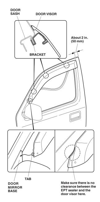
7. Check that the distance between the rear end of the door visor and front door is about 2 in. (50 mm).
