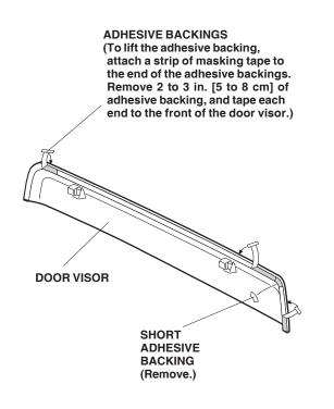
14. Push the two door visor brackets onto the door sash.
