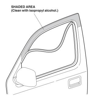
3. Locate the door sash in the area where the EPT sealer will attach. Using isopropyl alcohol on a shop towel, thoroughly clean the area.
