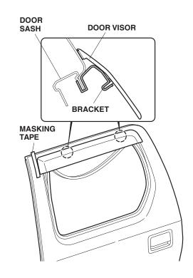
15. Align the front end of the door visor with the masking tape. While holding light pressure on the door visor, carefully remove the adhesive backing in the directions shown. Using the palm of your hand, hold the door visor firmly against the door for 30 seconds.
