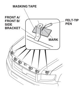
8. Using a felt-tip pen, mark the masking tape at the center of each bracket. Remove all of the brackets from the hood.
