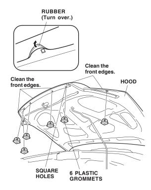
Clean the front edge of the hood with the other alcohol pad from the kit. Slide the front brackets A and B and the side brackets over the lip of the hood. Align the hole in each bracket with the hole in the plastic grommet.
