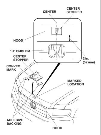
2. Remove the adhesive backing from the center stopper, and attach it to the hood at the marked location with the convex mark facing down.
