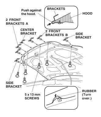
Install the center bracket over the hood around the protective tape. Push the center bracket against the hood while you install the screw.  Close the hood. Position the air deflector on the hood, and attach the air deflector to the two front brackets A, two front brackets B and center bracket using the five clips A.
