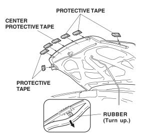
10. Attach the remaining protective tape around the center front edge of the hood. Remove the masking tapes.
