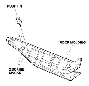
While wearing eye protection drill two holes on the roof molding at the holes made in step 2 with a 3 mm drill bit.
