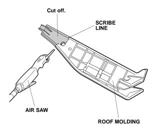
6. Remove the roof moldings by carefully lifting it upward from four vehicle roof molding clips.
