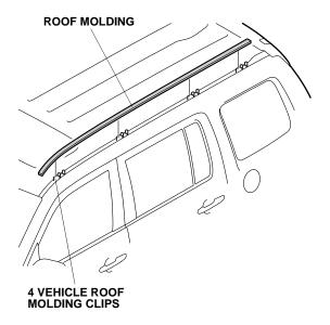
7. Remove and discard four vehicle roof molding clips from the roof molding or the stud bolt on the roof.
