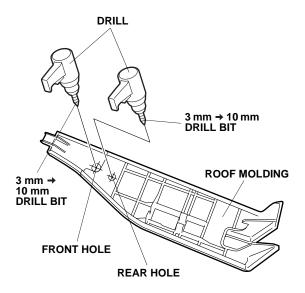
4. Widen the front and rear holes with a 10 mm drill bit.
