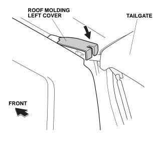
12. Reinstall the roof moldings back onto the roof of the vehicle with two new roof molding clips installed on step 11.
