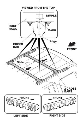
16. Tighten eight thumbwheel screws to secure the cross bars to the roof racks.
