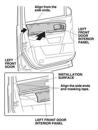
32. Press the left front door interior panel firmly to attach while removing the adhesive backings that you temporarily attached to the surface side.
