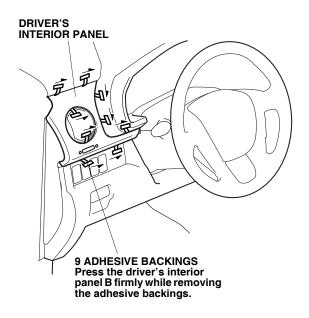
18. Using a rubber roller, apply pressure against the driver's interior panel B and roll from one end to the other.
