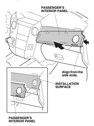
5. Press the passenger's interior panel firmly to attach while removing the adhesive backings that you temporarily attached to the surface side.
