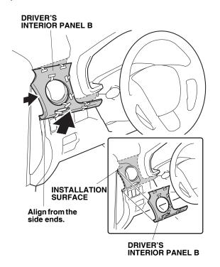
17. Press the driver's interior panel B firmly to attach while removing the adhesive backings that you temporarily attached to the surface side.
