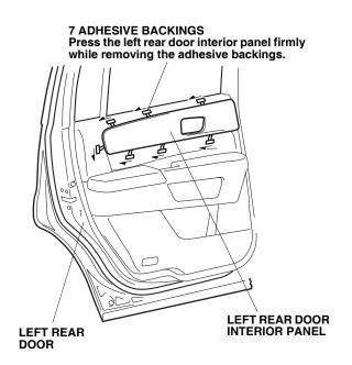
41. Using a rubber roller, apply pressure against the left rear door interior panel and roll from one end to the other.
