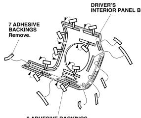
9 ADHESIVE BACKINGS Attach a piece of tape to an end. Peel back the adhesive backing partway and attach it to the surface side of the panel.
