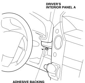
ADHESIVE BACKING Press the driver's interior panel A firmly while removing the adhesive backing. 12. Using a rubber roller, apply pressure against the driver's interior panel A and roll from one end to the other.
