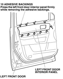
25. Using a rubber roller, apply pressure against the left front door interior panel and roll from one end to the other.
