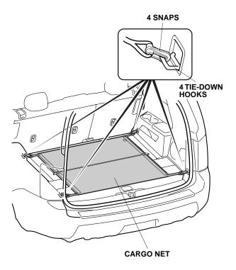
4. Attach four snaps of the cargo net to the four tie-down hooks in the cargo area.
