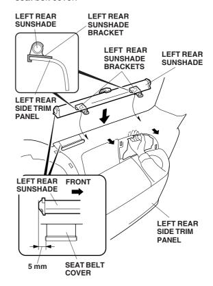
6. Using a felt-tip pen, mark the left rear side trim through the center of each bracket hole. Remove the rear sunshade.
