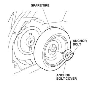
3. Pull away the weatherstrip from the left rear side trim panel. Remove the anchor bolt, disengage the three clips, and the four retaining tabs, and pull out the rear portion of the left rear side trim panel.
