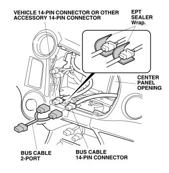
48. Plug the bus cable 14-pin connector into the audio-navigation unit or the audio unit, and reinstall the center panel.
