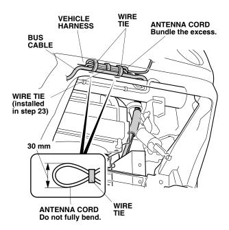
46. Secure the antenna cord and the bus cable to the vehicle harness with two wire ties. Do not bend the antenna cord more than 30 mm.
