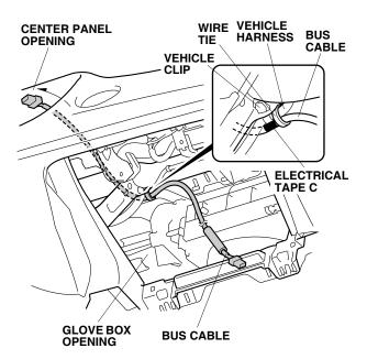
27. Secure the bus cable to the vehicle harness at masking tape C with one wire tie.
