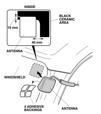
15. Remove four adhesive backings from the antenna, and attach the antenna to the windshield as shown. Firmly press the antenna against the windshield to ensure good adhesion. 16. Using isopropyl alcohol on a shop towel, thoroughly clean the outside of the windshield where the cover seal will attach. Remove the adhesive backing from the cover seal, and attach the cover seal to the windshield as shown.
