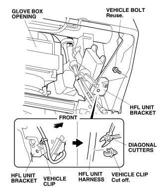
35. Remove the vehicle bolt from the HFL unit bracket.
