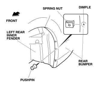
7. Install one spring nut over the pierced dimple on the rear bumper. Make sure to install the spring nut in the correct position and orientation.
