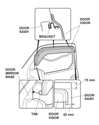
5. Adjust the location of the door visor so that the clearance between the door visor and door sash is 73 mm at the top, and 42 mm at the back. There should be no clearance between the door mirror base and the visor.
