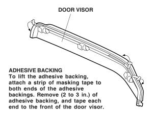
Insert the front tab of the door visor under the door mirror base, and attach the three brackets to the door sash.
