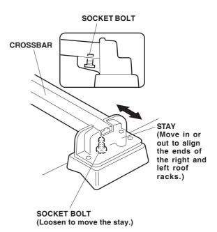
9. Temporarily tighten the 12 socket bolts and 12 washers.
