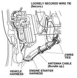
75. Using two wire ties, secure the antenna cable to the engine starter harness.
