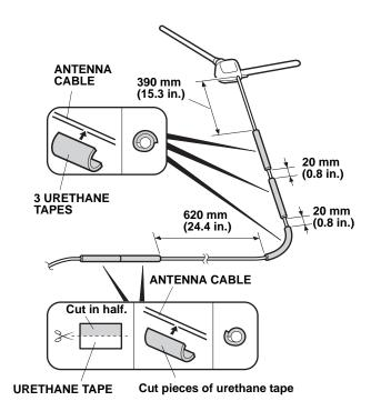
54. Cut one urethane tape in half. Wrap the two cut pieces around the antenna cable at the measurements shown.
