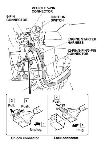
28. Unplug the vehicle 5-pin connector from the ignition switch, and plug the engine starter harness 5-pin connector into the ignition switch.
