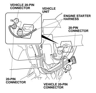
35. Align the green tape on the engine starter harness with the clip on the vehicle harness, and secure the engine starter harness to the vehicle harness using one wire tie.
