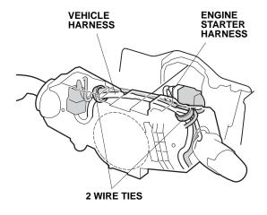
33. Using two wire ties, secure the engine starter harness to the vehicle harness in the areas shown.
