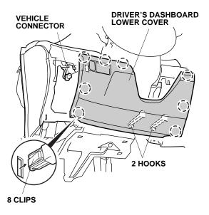
13. Remove the driver's dashboard under cover (three clips and one pin).
