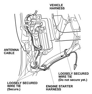
66. Secure the antenna cable using the three loosely secured wire ties.
