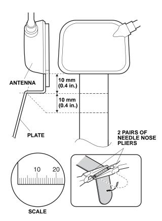
53. Starting near the antenna end of the cable, wrap three urethane tapes around the antenna cable at the measurements shown.
