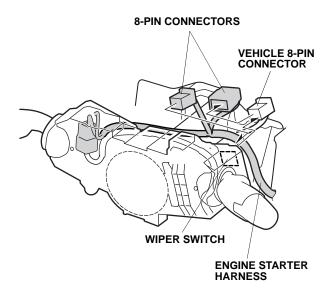
32. Using two wire ties, secure the engine starter harness to the vehicle harness. Do not secure to the SRS harness.
