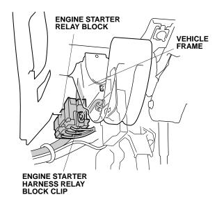
74. Bundle up the excess antenna cable and secure it to the engine starter harness and the vehicle harness using the loosely secured wire tie.
