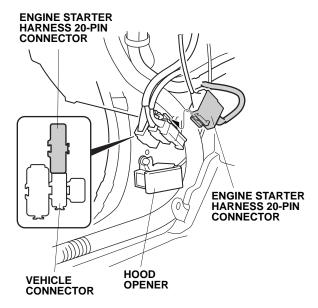
Remove and discard the hood opener bolt. Install the ground bolt with the engine starter harness ground terminal attached.
