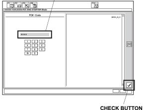
11. Check that "The registration of the Remote Control Engine Starter Unit has been completed" is shown, then click the check button.
