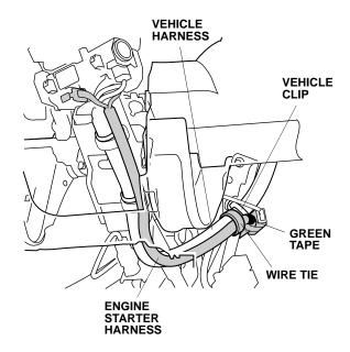
36. Near the connector, secure the engine starter harness to the vehicle harness using one wire tie.
