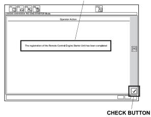
12. Check that "Check that the engine can be started by the Transmitter" is shown, then click the check button.
