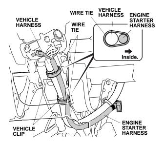
34. Unplug the vehicle 20-pin connector from the vehicle unit removed in step 21, and plug it into the engine starter harness 20-pin connector. Plug the remaining engine starter harness 20-pin connector into the vehicle unit.
