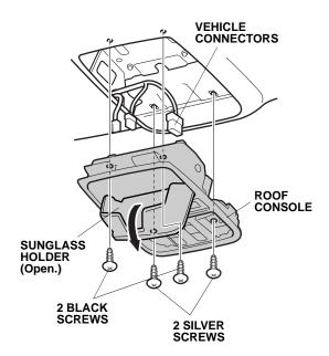
7. Turn the sunvisor holder 45° and remove the two sunvisor holders.
