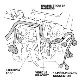
27. Route the 12-pin/8-pin/5-pin connector end of the engine starter harness to the ignition switch.
