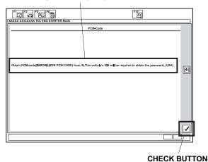
10. Input the PCM Code, then click the check button. NOTE: To ensure security, the PCM code (password) is changed everyday, so it is impossible to register the remote controlled engine starter if the date of the PCM code acquisition and registration are different. The date of the HDS tester should also be the same.
