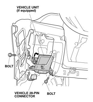
21. Remove the bolt, and remove the vehicle unit from the vehicle bracket.
