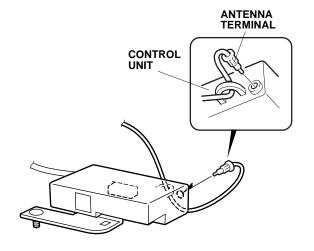
71. Secure the control unit to the vehicle frame using the flange nut.
