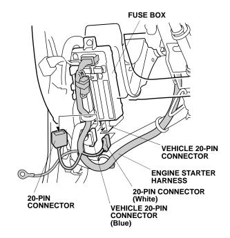
45. Attach the engine starter harness 20-pin connector to the vehicle connector as shown.
