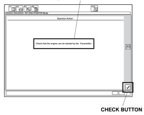
13. Perform the function test on next the page then remove the HDS.
