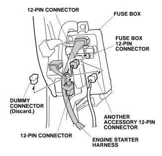
43. Using one wire tie, loosely secure the engine starter harness to the vehicle harness.
