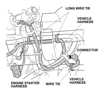
Using two long wire ties, secure the engine starter harness to the vehicle harness at the locations shown. 38. Reinstall the vehicle unit to the vehicle bracket using the bolt removed in step 21.
