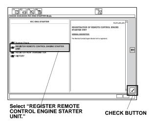
Check that "Obtain PCM-code (IMMOBILIZER PCM CODE) from iN. This vehicle's VIN will be required to obtain the password. (USA)" is shown, then click the check button.
