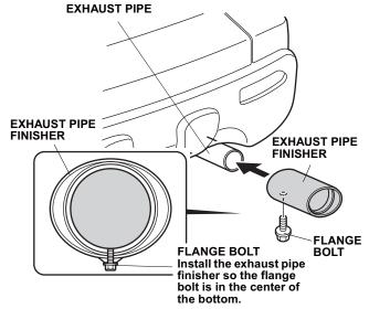
2. With the flange bolt on the bottom, slide the exhaust pipe finisher onto the exhaust pipe until it bottoms.
