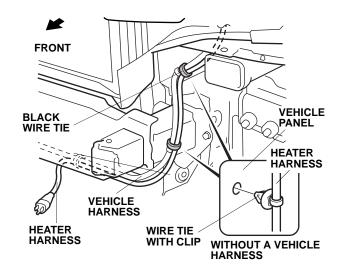
23. If the vehicle is not equipped with a vehicle harness, secure the heater harness to the vehicle panel using two wire ties with clip as shown.
