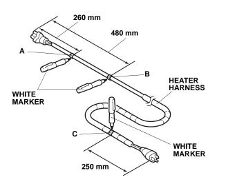
15. Plug the heater harness into the engine block heater.
