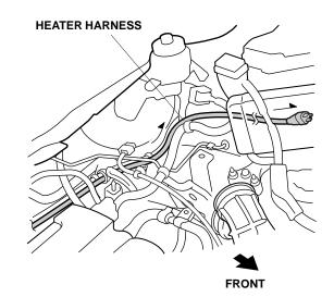
19. Route the heater harness through the engine compartment as shown.
