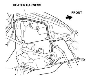
20. Route the heater harness through the front bulkhead as shown.
