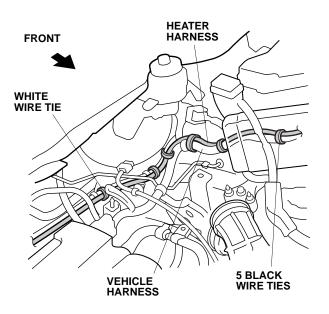
26. Secure the heater harness to the vehicle harness using two white wire ties in the areas shown.
