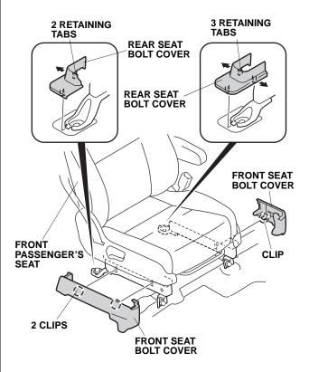
17. Remove the front seat bolt cover from the front passenger's seat (three clips).
