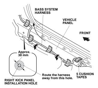
27. If the vehicle is equipped with an XM unit, secure the bass system harness to the vehicle panel using one cushion tape.
