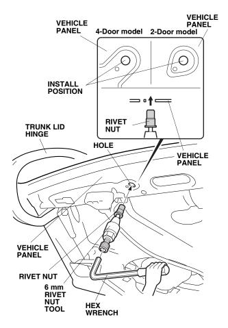
3. Holding the 6 mm rivet nut tool with the hex wrench, turn the 19 mm wrench clockwise and install the rivet nut to the vehicle panel.
