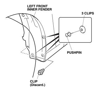
3. Using a pushpin, make small holes through the center of the three clips.
