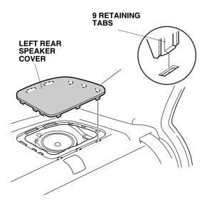
9. Remove the left rear speaker (one bolt and disconnect the vehicle connector).
