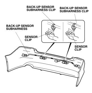
37. Using isopropyl alcohol on a shop towel, clean the bumper area where each harness tape will attach.
