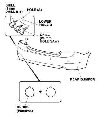
Using a 24 mm hole saw, enlarge the outboard (right and left corner sensor) bumper holes. On the driver's side, drill the lower 3 mm hole. On the passenger's side, drill the upper 3 mm hole.
