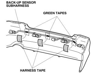
38. At each green tape location, secure the subharness to the rear bumper with harness tape.
