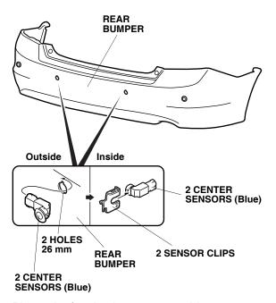
35. Plug in the four back-up sensor subharness 2-pin connectors into the backup sensors.
