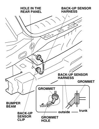
30. Attach the clip from the 8-pin connector into the hole in the rear panel.
