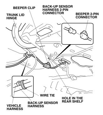
26. Secure the back-up sensor harness to the vehicle harness using one wire tie.
