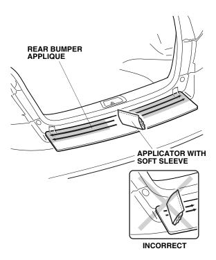
12. Once the flat surface is completely smooth with no bubbles, use the applicator with soft sleeve to apply the rear bumper applique to the rounded rear edge at the center as shown.
