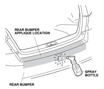
5. Remove the adhesive backing from the rear bumper applique.
