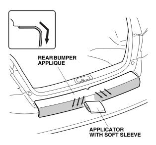
14. Remove the protective film from the top rear bumper applique. Slowly pull the protective film back as you go; do not pull it upward.
