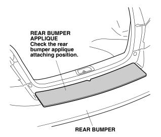
4. Using a spray bottle with protective tape application solution, spray the rear bumper where the rear bumper applique will attach.
