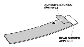
6. Using the spray bottle with protective tape application solution, spray the rear bumper applique.
