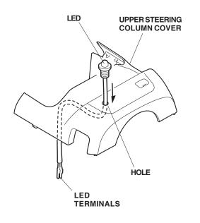
13. Get the 2-pin connector from the kit. Firmly push the LED terminals into the 2-pin connector until they click into position, then lower the lock.
