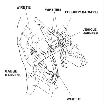
20. Position the upper steering column cover above the steering column, and plug the security harness 2-pin connector into the LED 2-pin connector.
