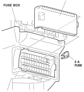
31. Attach the fuse label (OPTION FUSE 2 A) over the No.33 slot on the inside of the fuse box cover.
