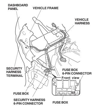
15. Route the security harness 2-pin connector along the vehicle harness, and route the security harness terminal between the vehicle frame and dashboard panel. 18. Remove the vehicle ground bolt, and attach the security harness ground terminal using this bolt.
