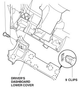
5. Using a tape measure and felt-tip pen, measure and mark the driver's dashboard lower cover.
