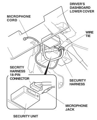
28. Fold the security harness and microphone wire, and secure it with one wire tie so that there is no tension applied to the microphone jack. 29. Fold the excess length of the microphone wire, and secure it to the vehicle harness with two wire ties.
