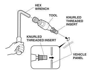
6. Holding the tool with the hex wrench, turn the 27 mm wrench clockwise and install the knurled threaded insert onto the vehicle panel.
