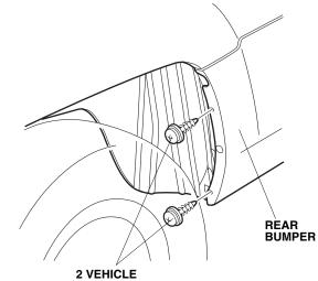
2 VEHICLE SELF-TAPPING SCREWS 2. Remove one vehicle clip from the left rear inner fender.
