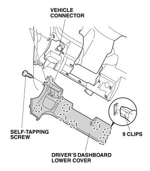
32. Remove the switch lid from the driver's dashboard lower cover, and install the switch to the driver's dashboard lower cover.
