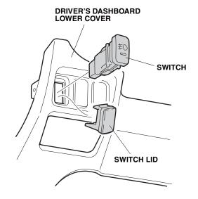
33. Unplug the vehicle 3-pin connector and plug the switch harness 3-pin connector into the vehicle 3-pin connector as shown.
