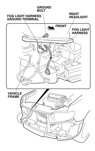
9. Secure the fog light harness ground terminal to the vehicle frame with one ground bolt.
