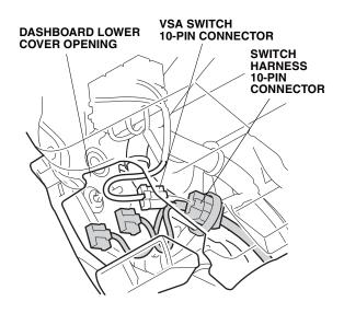
37. Plug the switch harness 10-pin connector (gray) into the fog light switch, and plug the switch harness 10-pin connector (gray) into the vehicle VSA switch.
