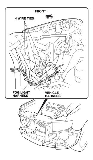
13. Secure the fog light harness to the vehicle harness with four wire ties.
