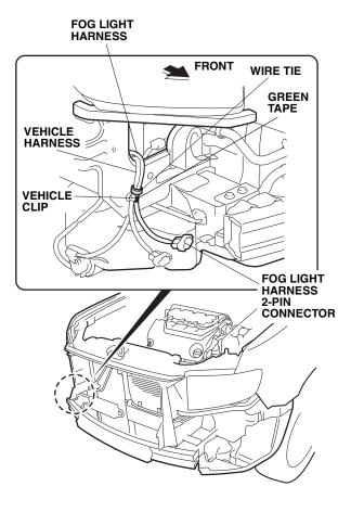
11. Secure the fog light harness to the vehicle harness with one wire tie.
