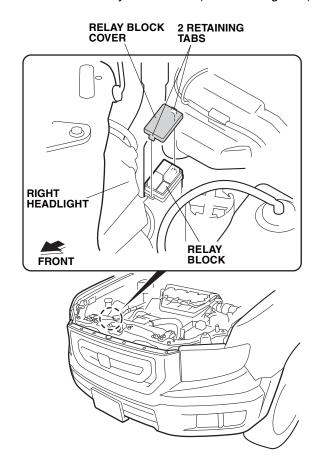
27. Install the relay into the vehicle relay block.
