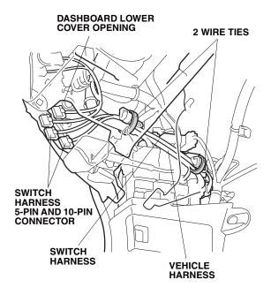
35. Secure the switch harness to the vehicle harness with two wire ties.
