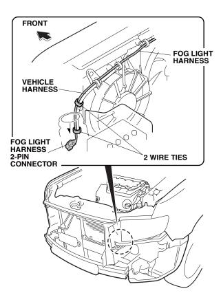
17. Secure the fog light harness to the vehicle harness with two wire ties.
