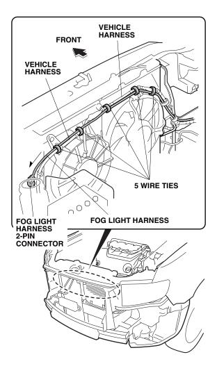
15. Secure the fog light harness to the vehicle harness with five wire ties.
