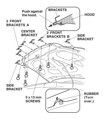
12. Install the center bracket over the hood around the protective tape. Push the center bracket against the hood while you install the screw.
