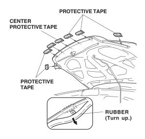
10. Attach the remaining protective tape around the center front edge of the hood. Remove the masking tapes.
