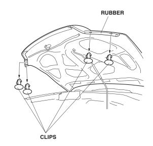
4. Turn over the rubber molding and locate the six square holes in the hood. Push one plastic grommet into each square hole.
