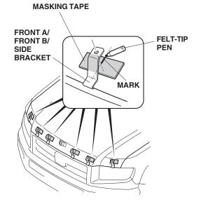
8. Using a felt-tip pen, mark the masking tape at the center of each bracket. Remove all of the brackets from the hood.
