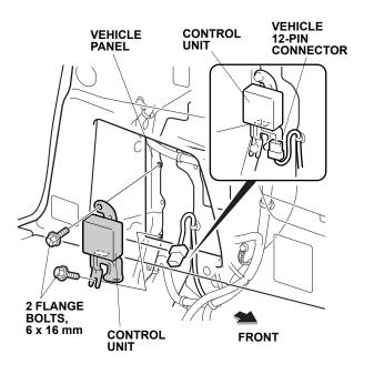
7. Plug the vehicle 12-pin connector to the control unit.
