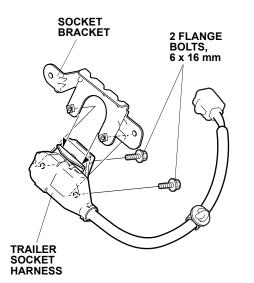
11. Secure the trailer socket harness to the vehicle frame with two 6 x 16 mm washer bolts.
