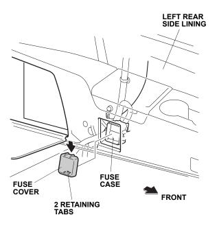
18. Plug the two 7.5A fuses and one 20A fuse to the fuse case.
