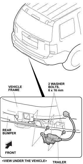
TRAILER SOCKET HARNESS 12. Release the vehicle 10-pin connector from the connector clip, and remove the dummy connector from the vehicle 10-pin connector.
