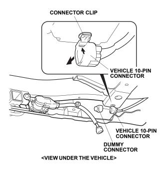
13. Plug the trailer socket harness 10-pin connector to the vehicle 10-pin connector.
