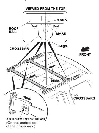
3. Tighten eight thumbwheel screws to secure the crossbars to the roof rails.
