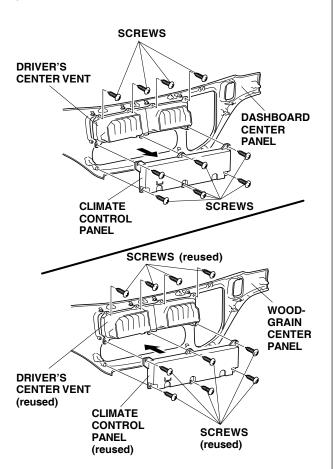
4. Remove the climate control panel (six screws), and transfer the control panel to the wood-grain center panel.
