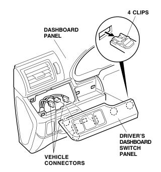
7. Remove the switch assembly (four screws), and transfer the switch assembly to the wood-grain switch panel.
