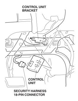
18. Plug the security harness 18-pin connector into the control unit.
