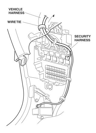
15. Continue routing the security harness along the vehicle frame, and secure it with one wire tie. Wrap one wire tie with clip around the security harness and attach the wire tie with clip to the hole in the vehicle frame.
