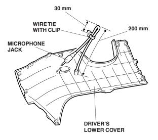
23. While holding the driver's lower cover near the dashboard, attach the wire tie with clip into the vehicle bracket.
