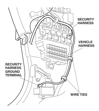
14. Route the security harness up along the vehicle harness, and secure it to the vehicle harness with one wire tie.
