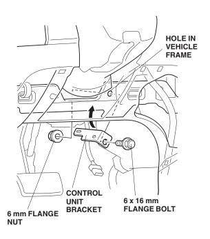
17. Install the control unit to the control unit bracket.
