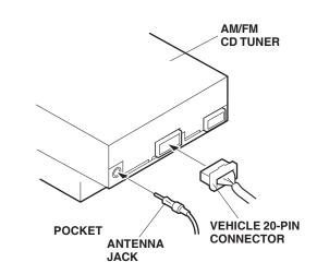
21. Connect the vehicle connectors to the center panel, and reinstall the center panel.
