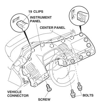
7. Remove the center panel from the instrument panel by releasing the four clips.
