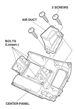
10. Loosen the four bolts on the right and left audio brackets.
