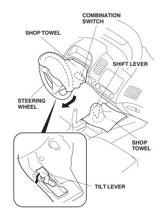
5. To protect the dashboard area, place a shop towel over the steering wheel and shift lever.
