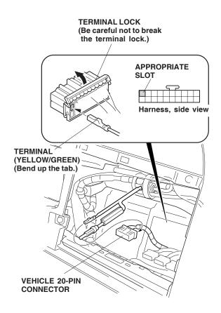
15. Carefully push the wire terminal (yellow/green) of the antenna subharness into the appropriate slot of the vehicle 20-pin connector. Reattach the terminal lock.
