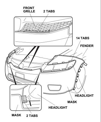
9. Pull the mask back toward the wheelwell, smooth out any wrinkles, and attach the five plastic hooks to the fenderwell, then bend the metal tab around the fenderwell. Repeat on the other side.
