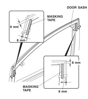
27. Using isopropyl alcohol on a clean shop towel, clean the area where the visor will attach.
