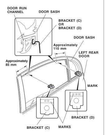
2. Install a bracket (C) and a bracket (D) on the door sash at the measurements shown. Verify the shape and the identification mark stamped on each bracket. Be sure to use the correct bracket at the proper location. 3. Position the left rear door visor on the door sash.
