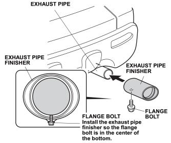
2. With the flange bolt on the bottom, slide the exhaust pipe trim onto the exhaust pipe until it bottoms.
