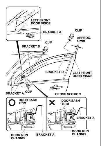
14. Position the left front door visor on the door sash by hooking the front bracket of the door visor on the door sash. Adjust the positions of bracket A and brackets D and install the three clips. Make sure there is no clearance between the bracket and door sash trim.
