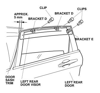
4. Attach masking tape to the left rear door visor at both ends of the door visor, then remove the left rear door visor (three clips).
