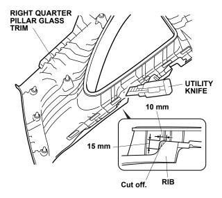
28. Using a ruler and a felt-tip pen, measure and mark the right quarter pillar glass trim in the area shown.
