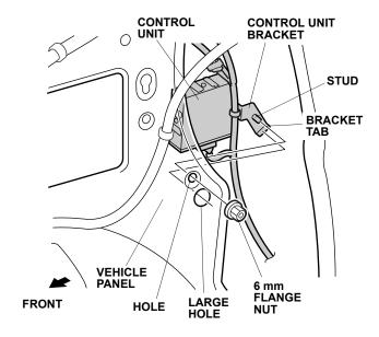
26. Install the back-up sensor harness clip into the hole in the vehicle panel.
