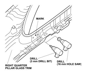
31. Using isopropyl alcohol on a shop towel, clean the right quarter pillar glass trim where the double-sided tape will attach. Remove the adhesive backing from the buzzer. Route the buzzer 2-pin connector through the 16 mm hole, and install the buzzer in the right quarter pillar glass trim with the two self-tapping screws. Install with the on/off switch and the volume control toward the front.
