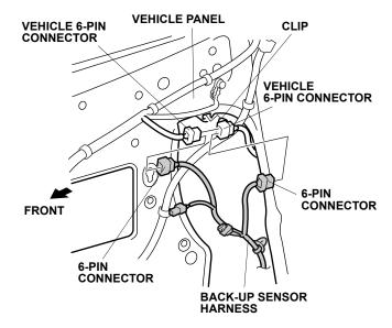
Plug the back-up sensor 6-pin connector into the vehicle 6-pin connector. Plug the other vehicle 6-pin connector into the other back-up sensor harness 6pin connector. 19. Reinstall the vehicle 6-pin connector clip to the vehicle panel.
