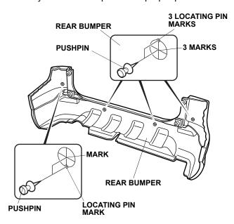
43. While wearing eye protection, drill a 3 mm hole at the eight pierced points you just made from the painted side of the rear bumper.
