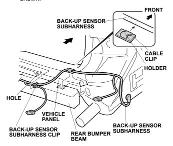
41. Route the back-up sensor subharness as shown. Attach the back-up sensor subharness clips into the holes in the vehicle panel.
