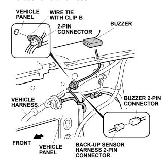
35. Secure the buzzer harness to the vehicle harness with one wire tie.
