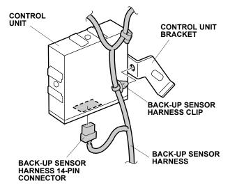
24. Attach the back-up sensor harness clip to the control unit bracket.
