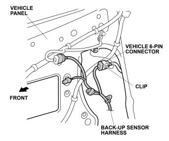
20. Secure the other 6-pin connector to the vehicle harness with one wire tie.
