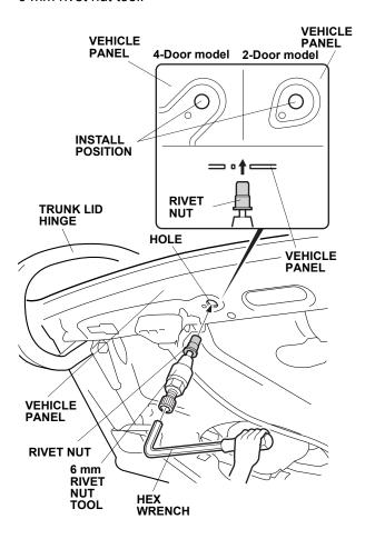
3. Holding the 6 mm rivet nut tool with the hex wrench, turn the 19 mm wrench clockwise and install the rivet nut to the vehicle panel.
