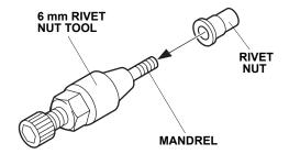
2. Open the trunk lid. Insert the rivet nut into the hole in the vehicle panel, and install the hex wrench on the 6 mm rivet nut tool.
