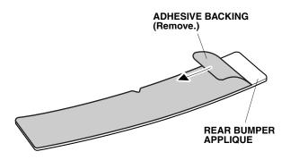
6. Using the spray bottle with 3M protective tape application solution, spray the rear bumper applique.
