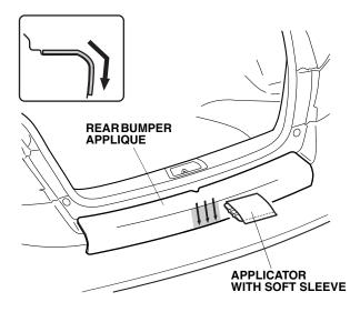
13. Use the applicator with soft sleeve to apply the rear bumper applique to the rounded rear edge on the left side as shown. Start in the middle and work outward. Repeat for the right side.
