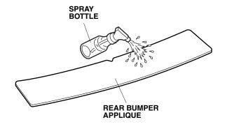
7. Align the V-notch of the rear bumper applique with the center of the trunk lid anchor as shown. Smooth rear bumper applique along the rear bumper and tape each end at the curved surface.
