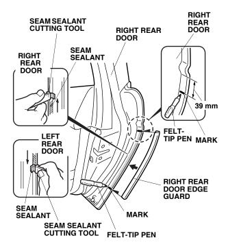
Position the cutting edge of the seam sealant cutting tool against the right rear door edge, and trim the seam sealant from mark to mark.
