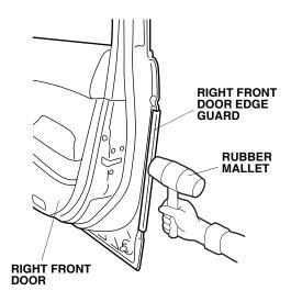
8. Repeat steps 3 through 7 to install the left front door edge guard.
