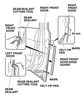
5. Position the cutting edge of the seam sealant cutting tool against the door edge, and trim the seam sealant from mark to mark.
