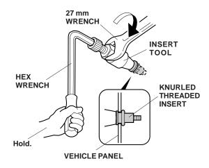
7. Remove the tool from the knurled threaded insert by turning the hex wrench counterclockwise.
