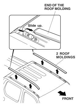
3. Remove the six clips from the roof channels.
