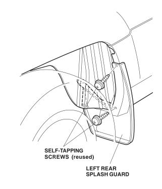
5. Repeat steps 1 thru 4 to install the right rear splash guard on the right side of the vehicle.
