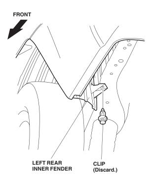
3. Position the left rear splash guard on the left rear inner fender and install the clip from the kit.
