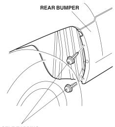
SELF-TAPPING SCREWS (Reuse.) 2. Remove and discard the clip from the rear of the left rear inner fender.
