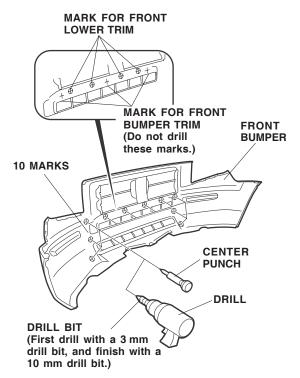
11. Get the left front bumper trim. While wearing eye protection, drill a 3 mm hole through the mark on the inside of the left front bumper trim.
