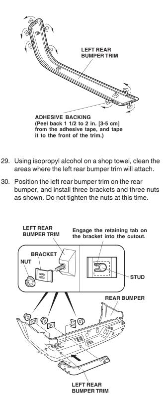
31. Align the upper line of the bumper trim with the masking tape. While holding light pressure on the trim, carefully remove the adhesive backings from the trim. After removing the adhesive backings, hold the trim firmly against the rear bumper with the palm of your hand for 30 seconds.
