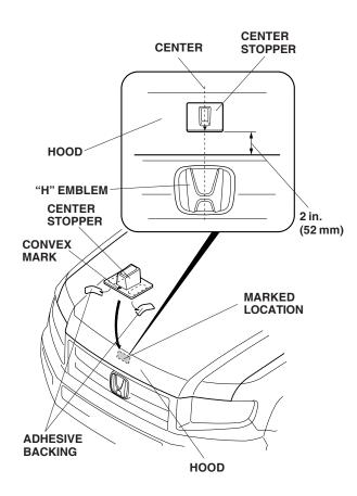
2. Remove the adhesive backing from the center stopper, and attach it to the hood at the marked location with the convex mark facing down.
