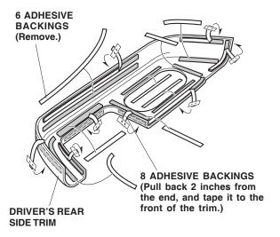
9. Position the driver's rear side trim on the existing panel. While holding pressure on the driver's rear side trim, carefully remove the adhesive backings from the driver's rear side trim. Hold the driver's rear side trim firmly against the panel with the palm of your hand, particularly at the edges. Remove all remaining adhesive backings from the driver's rear side trim.
