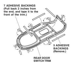
7. Position the rear door switch trim on the existing panel. While holding pressure on the rear door switch trim, carefully remove the adhesive backings from the rear door switch trim. Hold the rear door switch trim firmly against the panel with the palm of your hand, particularly at the edges.
