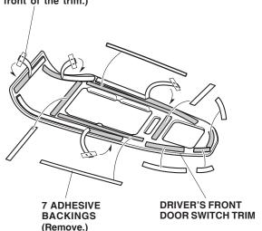
3. Position the driver's front door switch trim on the existing panel. While holding pressure on the driver's front door switch trim, carefully remove the adhesive backings from the driver's front door switch trim. Hold the driver's front door switch trim firmly against the panel with the palm of your hand, particularly at the edges.
