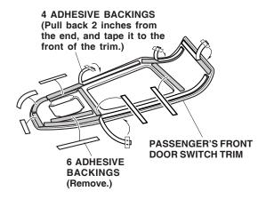
5. Position the passenger's front door switch trim on the existing panel. While holding pressure on the passenger's front door switch trim, carefully remove the adhesive backings from the passenger's front door switch trim. Hold the passenger's front door switch trim firmly against the panel with the palm of your hand, particularly at the edges.
