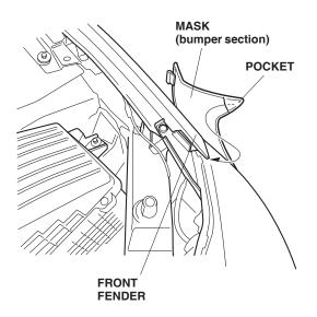
5. Attach the plastic hook from the bumper section to the vehicle frame. Fit the mask across the bumper, and attach the mask to the other side the same way.
