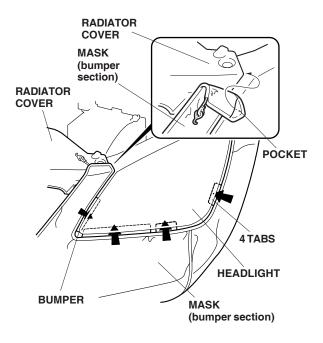
8. Secure two elastic straps on the bumper mask to the radiator cover as shown.
