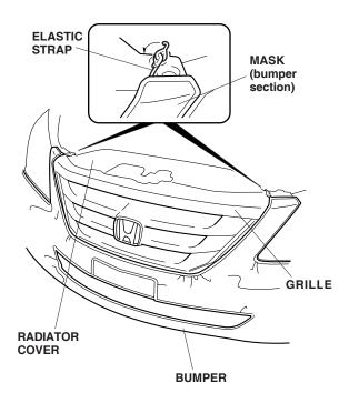
9. Attach four elastic straps to the inside top edge of the bumper opening, and attach five elastic straps to the bottom inside edge of the bumper opening as shown.
