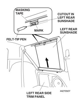
12. Using isopropyl alcohol on a shop towel, clean the left rear window above the marks you made on the masking tape.
