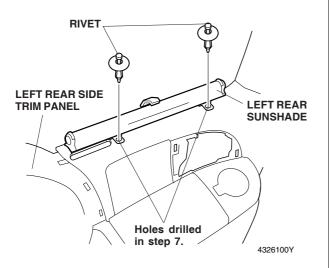
9. Secure the two brackets from the left rear sunshade to the left rear side trim panel with the two rivets. Reinstall the left rear side trim panel.
