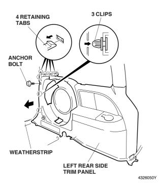
4. Remove the left speaker cover (two clips and three retaining tabs).
