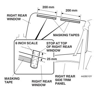
23. Pull up the rear sunshade until the cutouts in the sunshade reach the masking tape. Using a felt-tip pen, mark the top of the masking tape at each side of each cutout. Roll down the rear sunshade.
