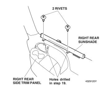
21. Secure the rear sunshade to the rear trim panel using two rivets from the kit, then reinstall the rear trim panel.
