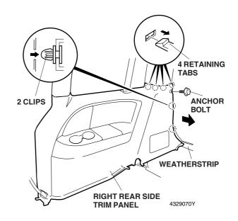
16. Remove the right rear speaker cover (two clips and three retaining tabs).
