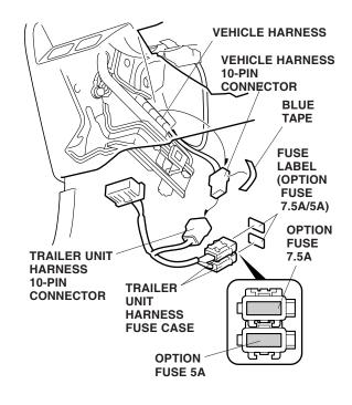
18. Install the trailer unit harness fuse case by sliding it onto the vehicle harness coupler holder.
