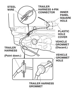
8. Remove the steel wire from the trailer harness 4pin connector. 9. Install a wire tie with clip to the 4-pin connector of the trailer harness. Remove the blue tape to free the 4-pin connector of the vehicle harness in the cargo area. Remove the dummy connector from the 4-pin connector of the vehicle harness and connect the 4-pin connector of the trailer harness. Secure the connected 4-pin connectors with a wire tie with clip to the vehicle harness and wrap an EPT sealer around it.
