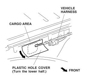
7. Remove and discard the rear left grommet from the body. Attach a piece of steel wire to the trailer harness 4-pin connector and route the 4pin connector through the vehicle grommet hole and into the hole in the cargo area. Seat the trailer harness grommet in the vehicle grommet hole with the end facing down.
