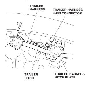
30. Install the connector bracket on the trailer harness 4-pin connector, and secure them to the trailer hitch with the flange bolt and flange nut. Route the trailer harness above the trailer hitch.
